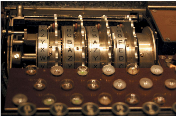
A U-Boat Enigma machine showing the internal Rotors
